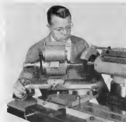
Figure 69A Motor Drive Equipment for Cylindrical Grinding Operations. Convenient for Grinding Tracer Fingers
